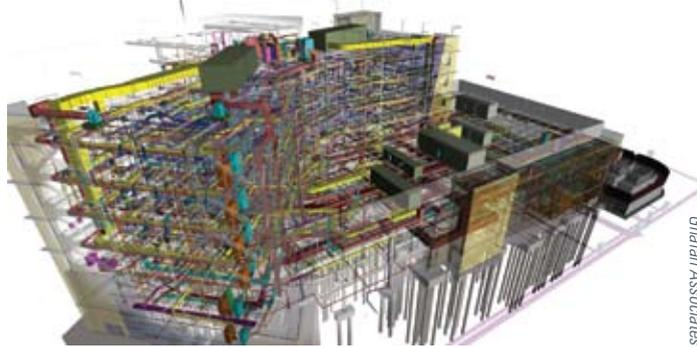
Detailed 3D modeling was required to coordinate systems before fabrication and construction.
